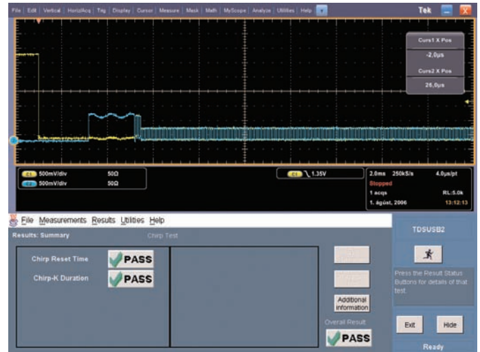
Figure 6. Test parameters for a CHIRP test.
