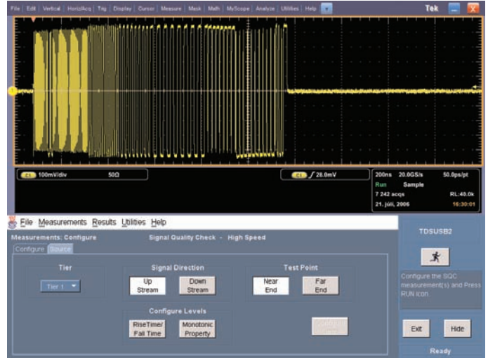
Figure 2. TDSUSB2 compliance test package running on a DPO7254.
