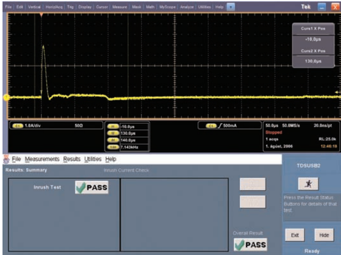
Figure 4. Illustration of a sharp intake of current using a DPO7254C.
