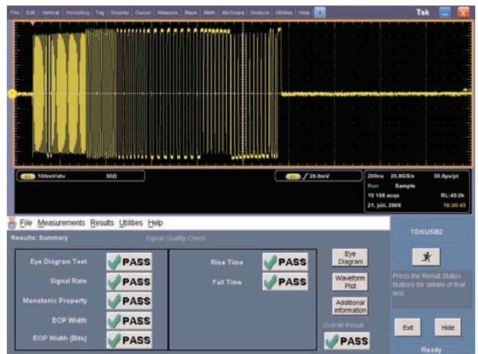
Figure 3. Measurement results are automatically displayed using the TDSUSB2 compliance test package.
